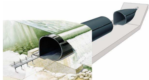
Figure 3. Schematic of Bridgestone Inflatable Dam
