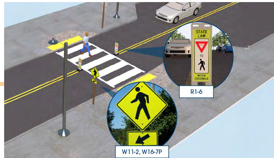
FIGURE 20. CROSSWALK VISIBILITY ENHANCEMENTS
